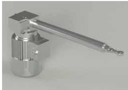
■ The electromechanical actuator is invaluable when a high degree of positioning precision is required, with the facility for optional position control (electrical signal - reading equipment is not provided). Applications on fans with maximum pressure of 10000 Pa; above this value non-standard actuator sizes must be specified (consult MZ Aspiratori for information).
